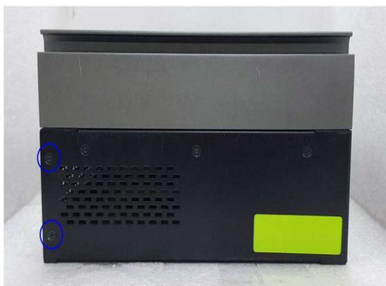
Step 12. fix the 8 screws on the system
