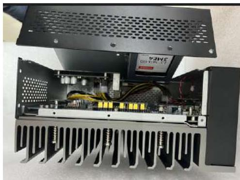
Step 11. fix the 2 screws on the system
