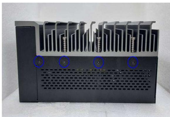
Step 2. Loosen the 8 screws on the system
