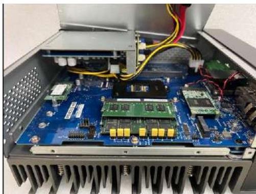
Step 5. Install DDR4 SO DIMM Memory Module on the system
