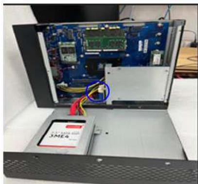
Step 6. Loosen the screw on the case
