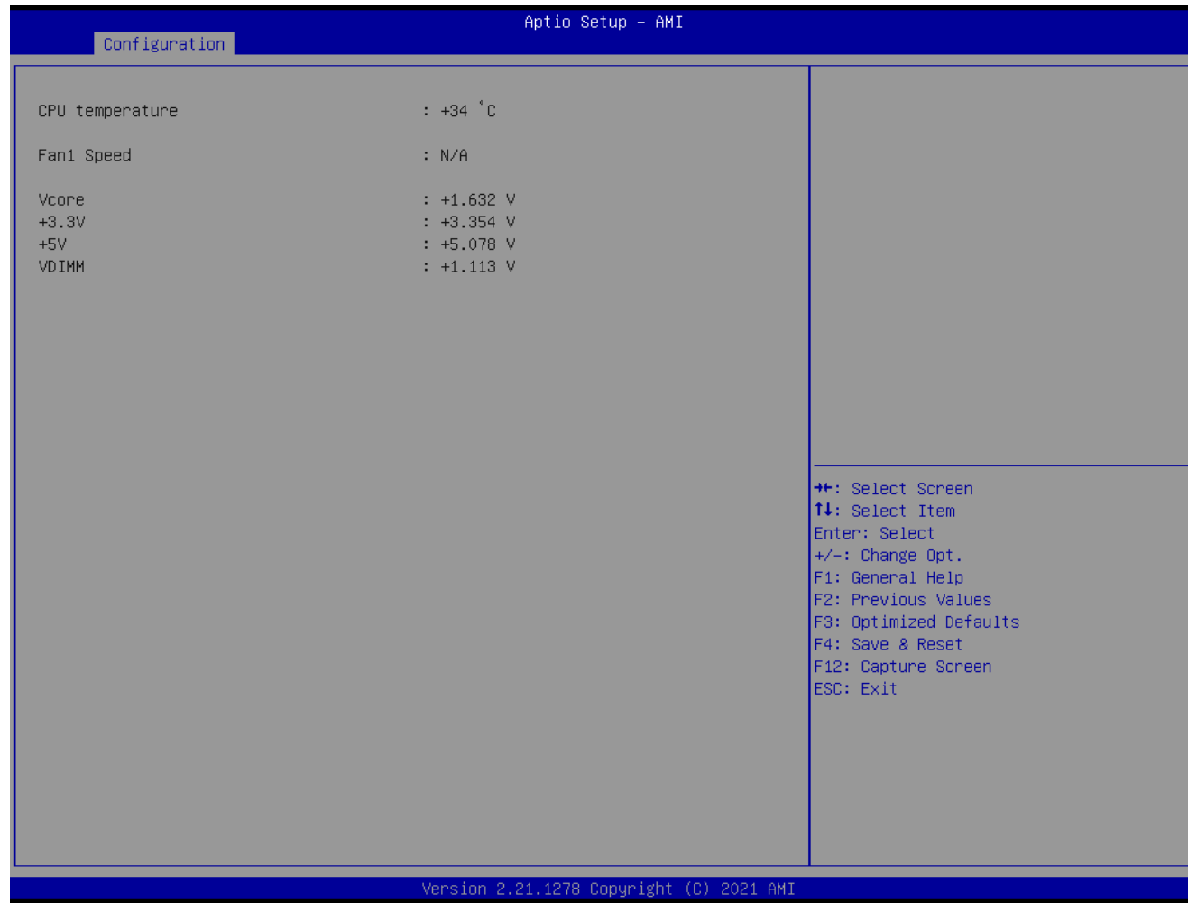
Figure 26 BIOS - Configuration - H/W Monitor
