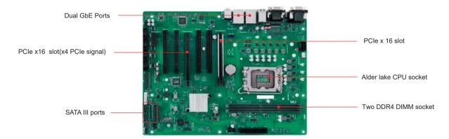
RUBY -D813 is based on Intel® H610E chipset and Desktop processors including Intel® 12 th Gen Core™ i3/i5/i7/i9 Sku. This board suppots DDR4 ,PCIe, and SATAIII. Those features help you to build high performance and stabile system.
