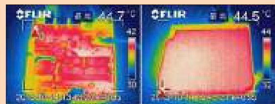
Thermal image of NANO-6060 M/B
