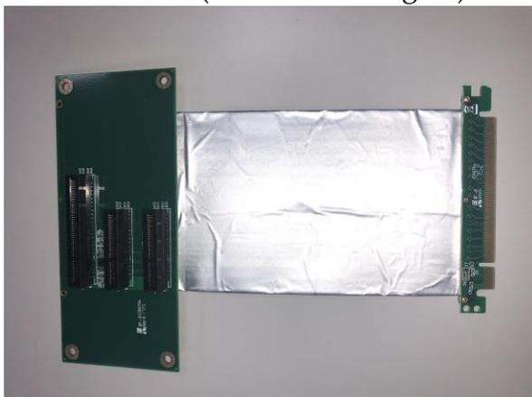
Install PCIe/PCI add-on card on 2x PCIe x4 riser card or 1x PCI and 1x PCIe x4 riser card.
