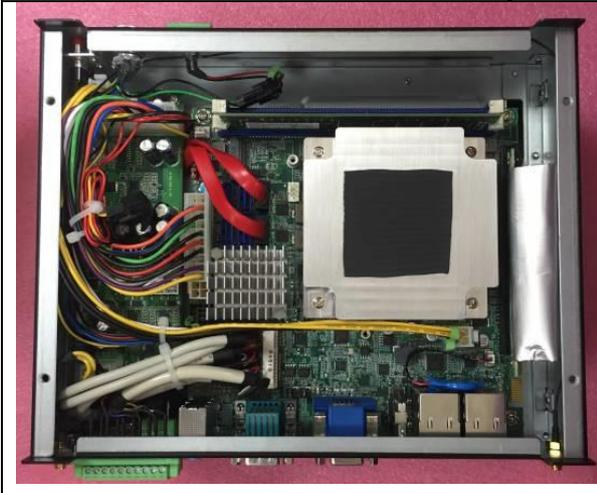
Step12. Fixed the screws of top heatsink (there are 4 screws)
