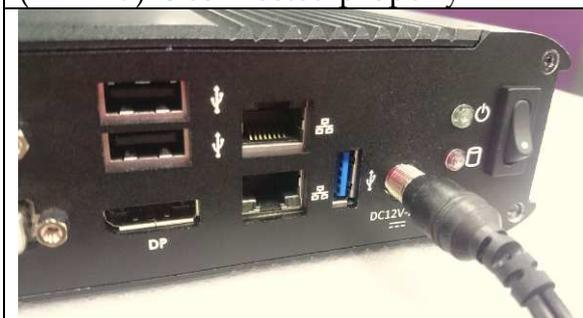
Step 2. Press the power switch to turn on the system
