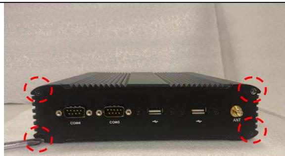
Step 2. Loosen the 4 screws of the rear cover
