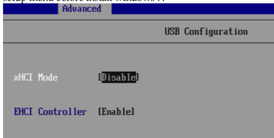
**Step2.** After complete the Windows 7 installation then change the BIOS setting of
