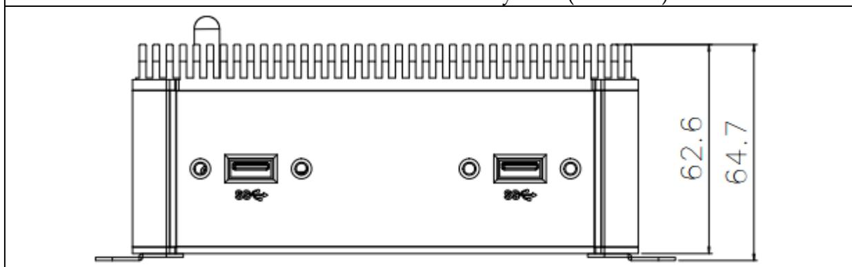
Front view of the WEBS-21A0 system (with optional kit: addition 2x USB 3.0)
