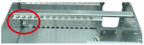
• 2U or 1U chassis: a mental bracket on the bottom of chassis to balance and support SBC from bending.
