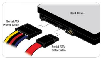
ROBO-6912VG2AR can support two (J10/J12) SATA interface (SATAIII, 6.0Gb/s) one mSATA (J22) interface on board; The SATA interface shall support 1.5Gb/3.0Gb & 6.0Gb operation per the SATA specification.
