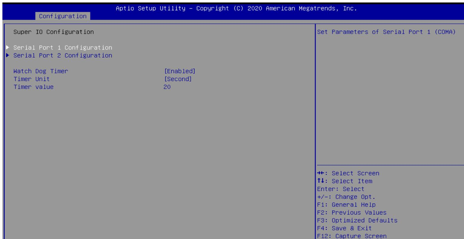
Figure 24 BIOS Super IO Configuration
