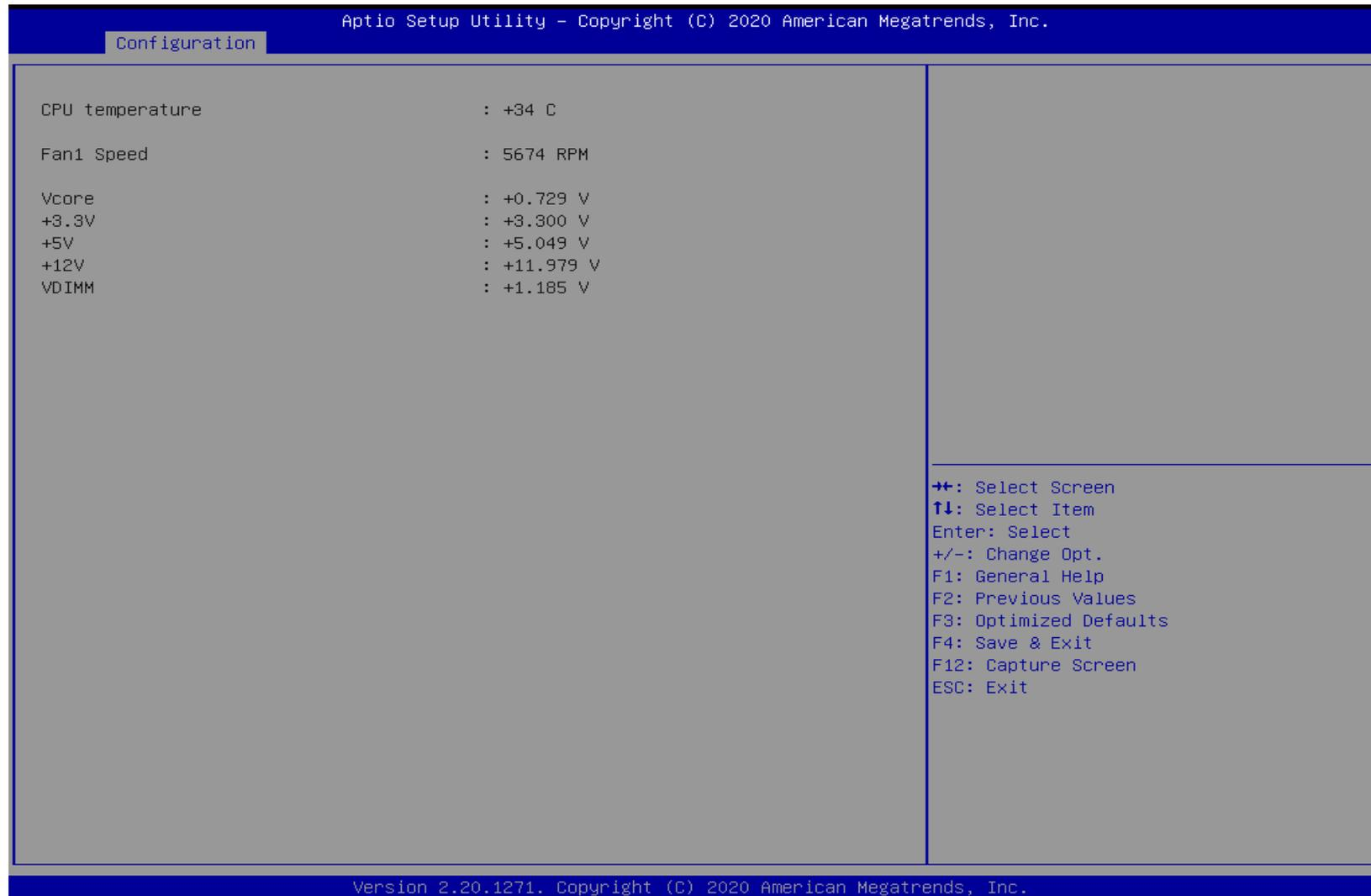
Figure 27 BIOS H/W MONITOR
