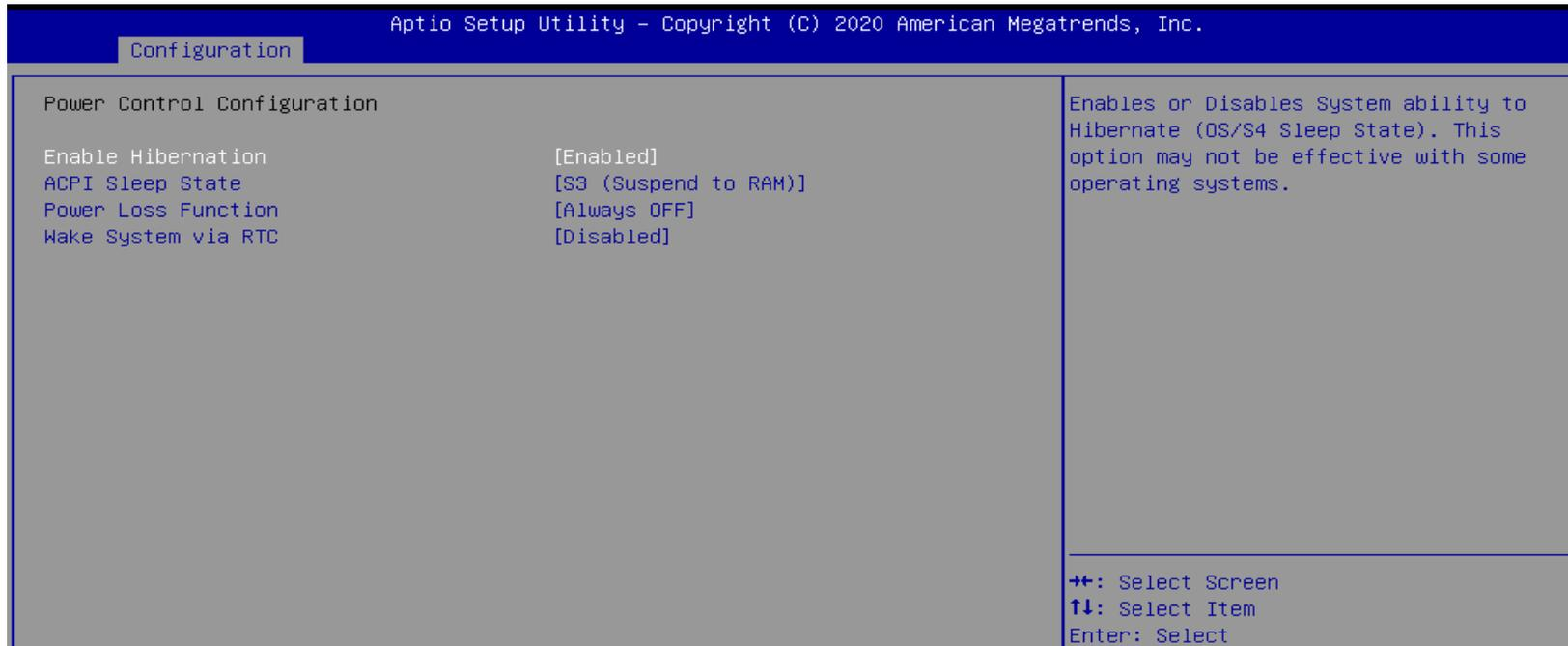
Figure 17 BIOS Power Control Configuration
