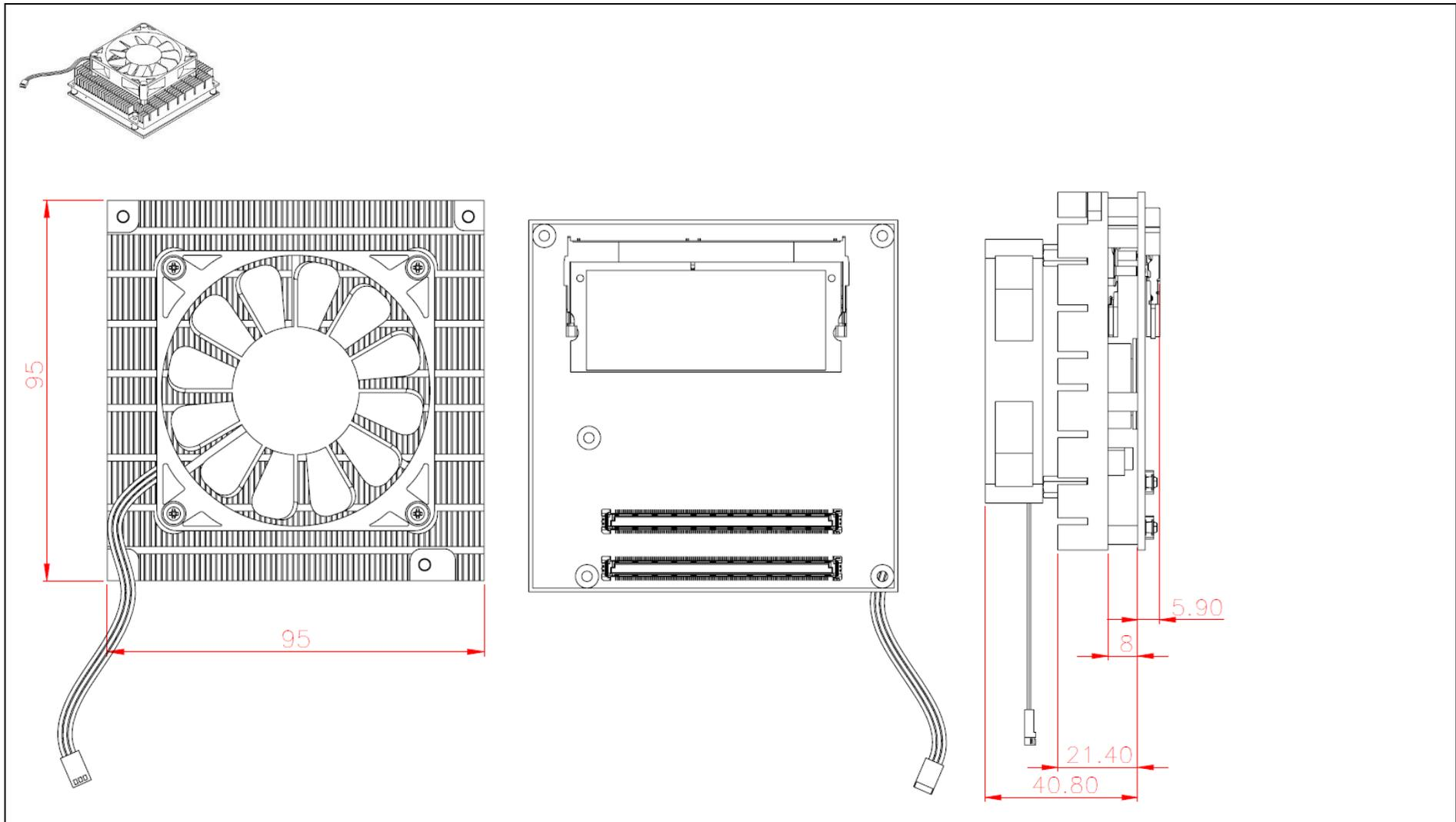
Figure 7 Heat sink / cooler mechanical dimensions
