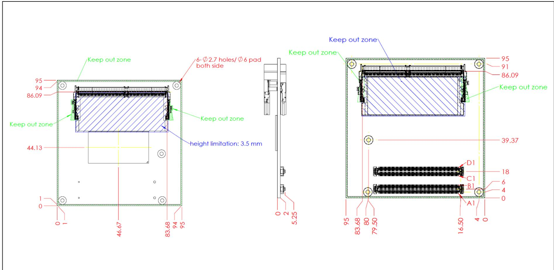
Figure 4 Mechanical Dimensions - Top & BOT & Assembly
