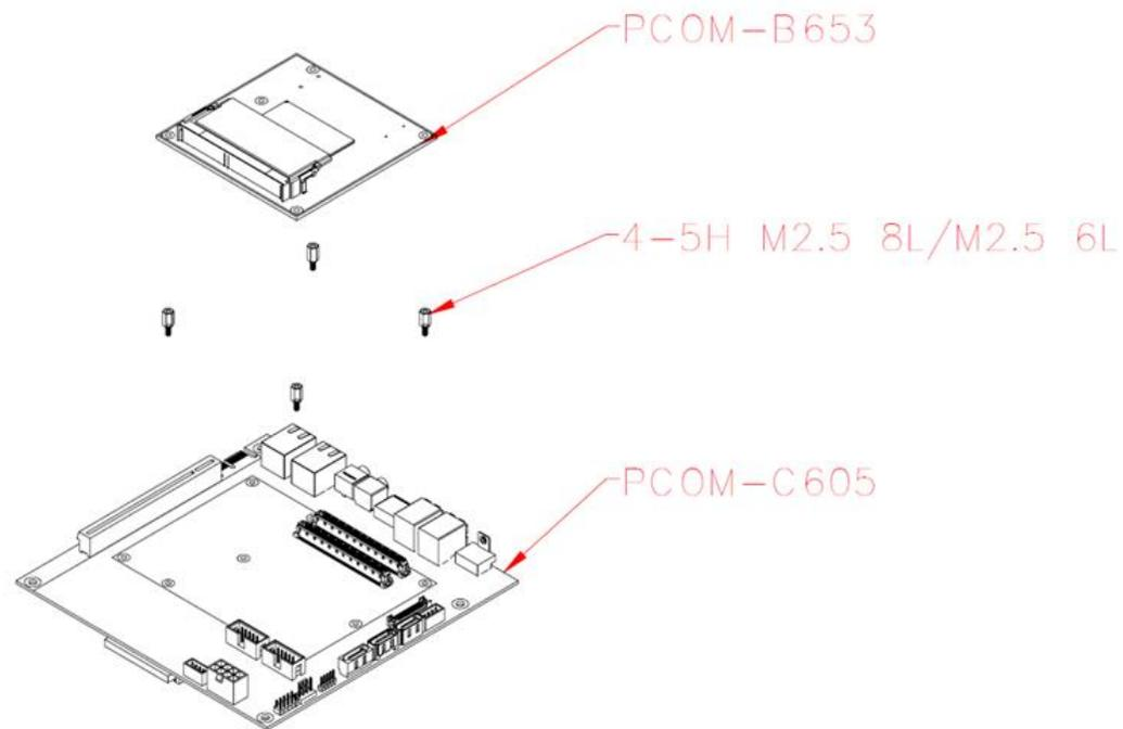
Figure 41 Assembly Step 1
