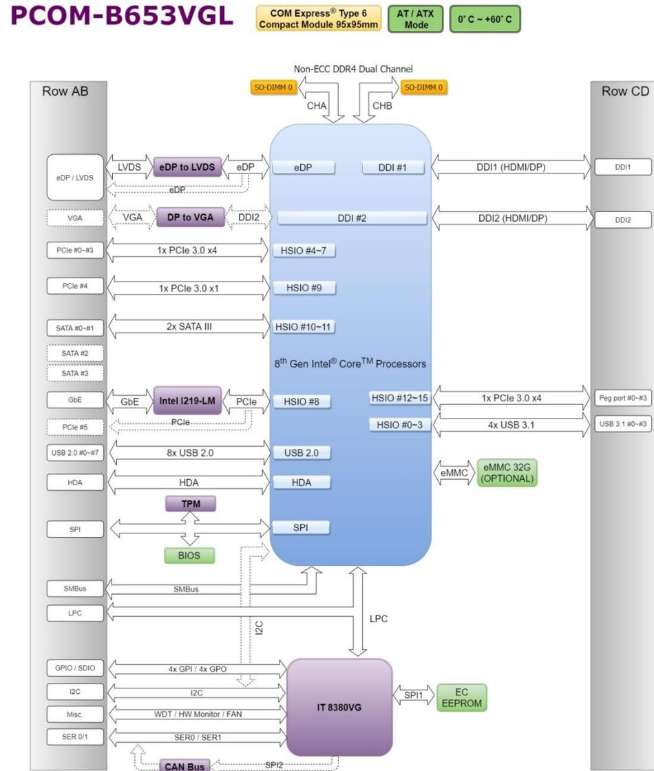
Figure 1 PCOM-B653VGL Block Diagram
