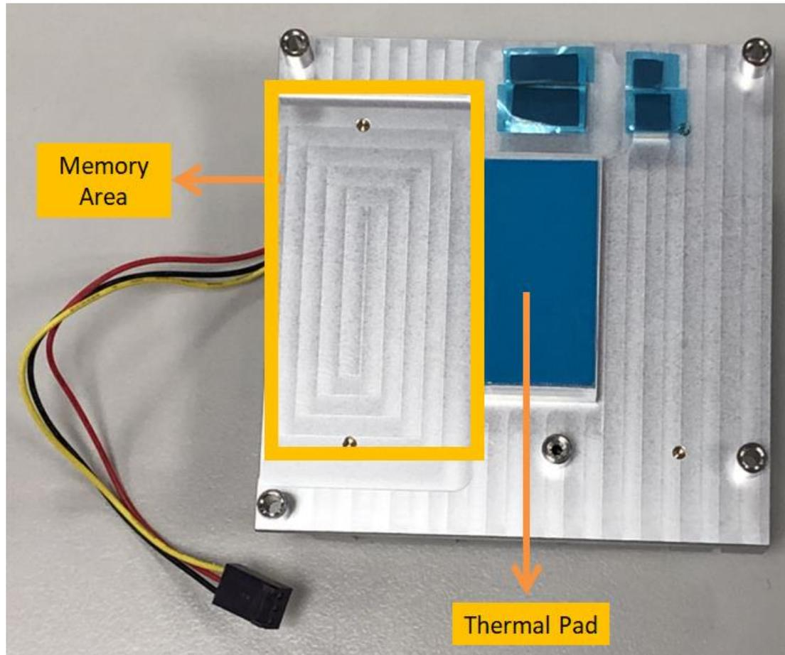
Figure 36 Cooler - Bottom
