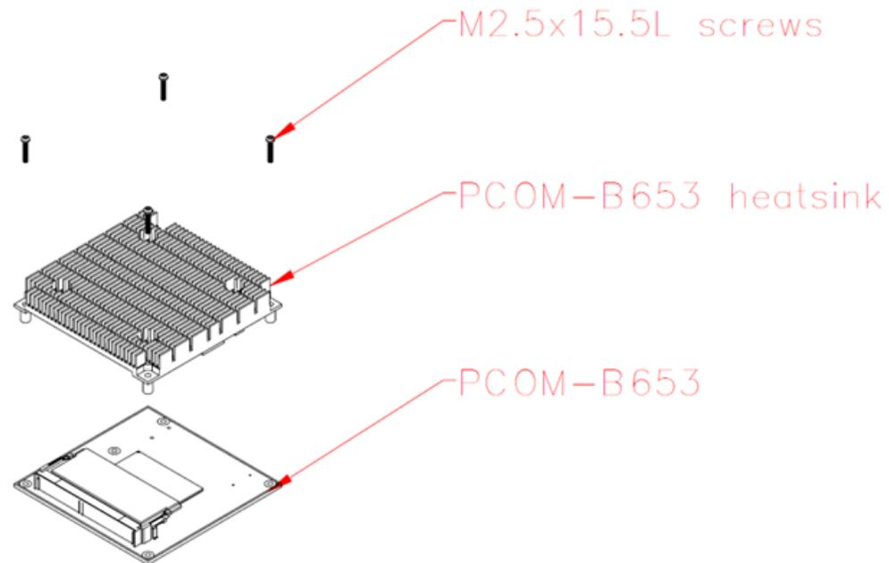
Figure 42 Assembly Step 2
