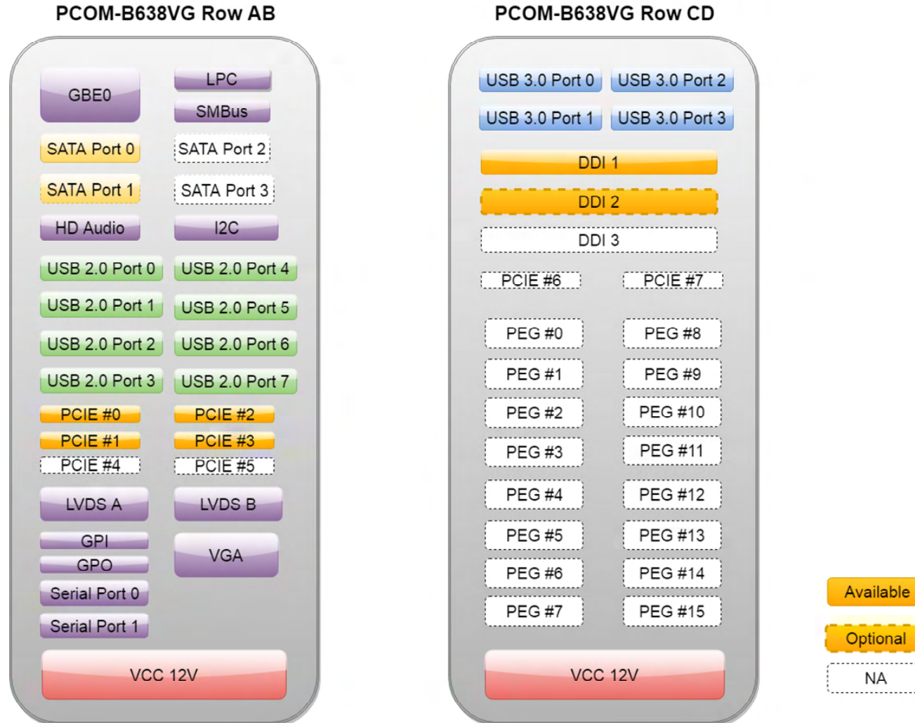
Figure 11 AB & CD Row connector signals
