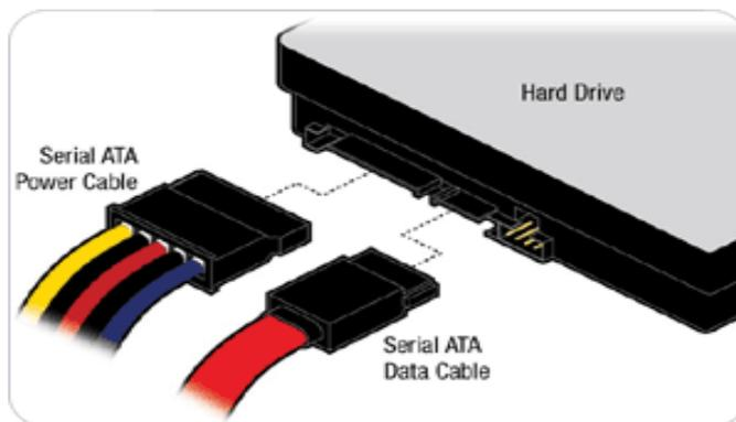
The PCOM-B632 can support two SATA interface (SATAII, 3.0Gb/s) to the PCOM-C600 carrier board with AHCI or IDE mode. It has two J28 & J30 SATA ports in PCOM-C600 carrier board.
