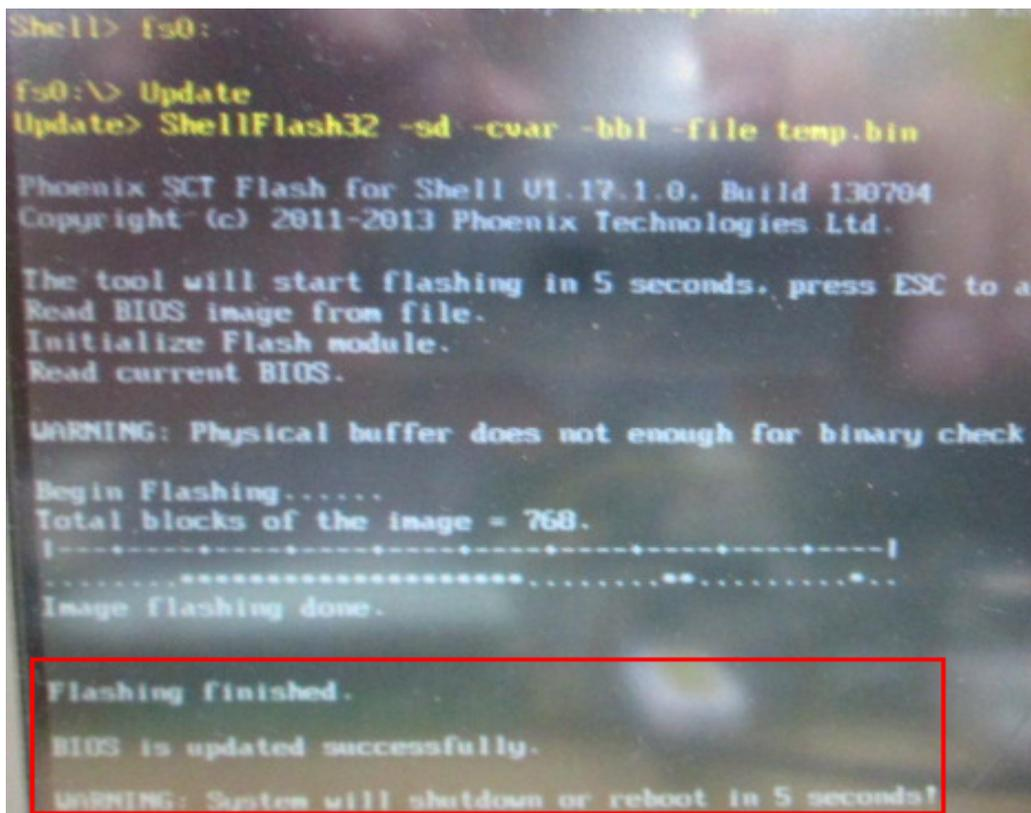
10. Please press the “F2” key to BIOS setup menu to select “Load Setup Defaults” and then select “Exit Saving Changes” option to finish all BIOS flash processes.
