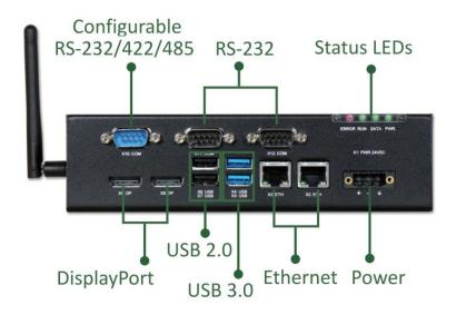
After mounting KUBE IPC, make any necessary cable connections.
