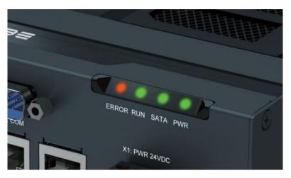
Four LEDs are provided on the KUBE IPC. These LEDs provide operating information
