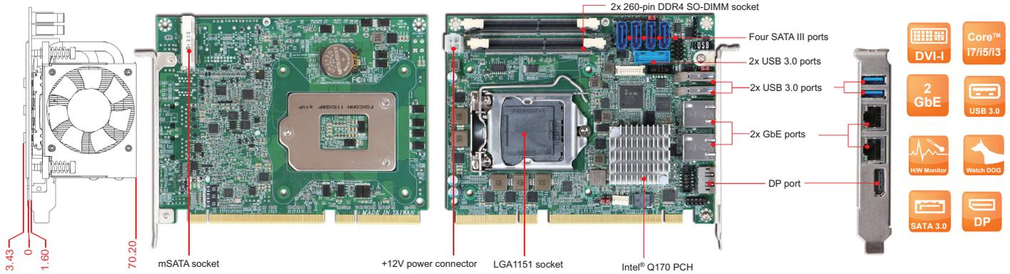
ROBO-6911VG2AR is based on Intel® C236/ Q170 chipset to support both Intel® Xeon® and Core™ i3 processors. Built with flexible PCI express expansions, ROBO-6911VG2AR is suitable for Medical, Industrial automation, and Digital Signage application.
