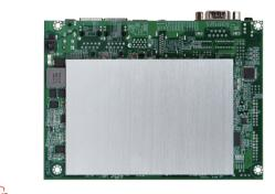
PEB-2773 build with Intel® Atom® processor E3900 series. Not only does it operates with TDP under 12W for fan-less applications, but it also supports industrial temperature range from -40°C to 85°C and wide voltage of power input from 12V to 24V.
