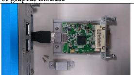
Step 6. Install the tray of graphic module back onto the system
