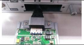
Step 5. Connect the cable to graphic module with which you want to replace and lock it
