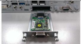
Step 7. Screw the tray of graphic module properly
